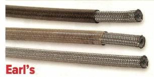
We've seen Earl's product all over race cars, and for good reason. They have an extensive line of hoses, fittings, and adapters to complete your fuel system. They recommend using their Speed-Flex hose for E85. It's got an extruded Teflon liner with a stainless steel outer braid. It comes in AN sizes -3 through -8, and is even resistant to brake fluid.
