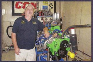
At 512 ci, the RM Competition Entry was the largest engine in the contest, making over 625 horsepower and nearly 600 lb-ft of torque.
