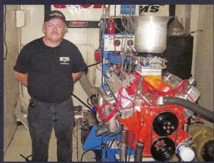
Known for making power, JD Engine and Machine made a strong statement as their nearly 500ci low-deck made a contest leading 724.5 horsepower.
