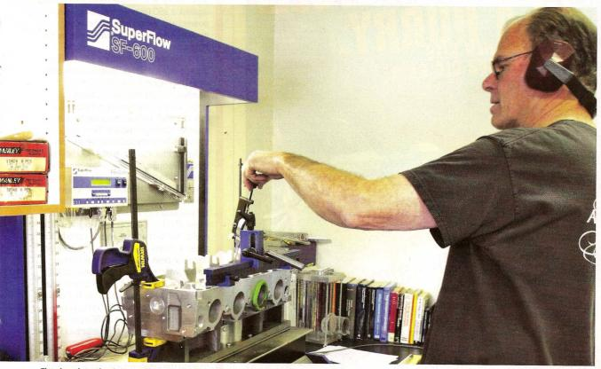
Flow bench testing is an easy way to discover how bore size affects airflow and performance. If you want to increase the airflow of even a simple small-block Chevy cylinder head, just change the test bore size adapter from the 305's 3.735-inch diameter to something like the 400's stock 4.125-inch bore. This could be worth 10 cfm at max flow. If you watch closely when cylinder head companies state their flow numbers, the smart ones will use a larger bore to improve the flow numbers.
