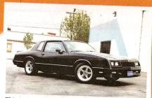
This is the Monte we just completed that now sits on 17x8 Center Lines with 41/2 inches of backspacing along with a set of 245/45R17 General Tire UHP Exclaim tires. The suspension is all Edelbrock.
