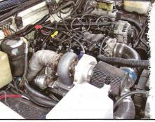
We ran across Bervil Hillis and his '94 Chevy 1500 pickup at the LS Fest. What makes his truck special is that '94 LS1 Corvette engine spooled up with a 67mm turbocharger that he bought used from an STS turbo system. Then Bervil made his own steel passenger-side exhaust manifold to mount the turbo. It makes for a great tow package.
